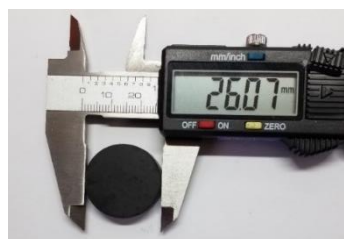
Figure 4 Appearance and dimensions of a sintered membrane
