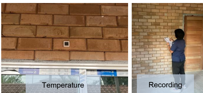
Figure 11 Temperature recording of a house built with interlocking blocks containing para-wood ash.
