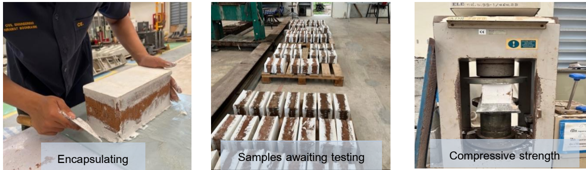
Figure 3 The compressive strength test of interlocking blocks.
