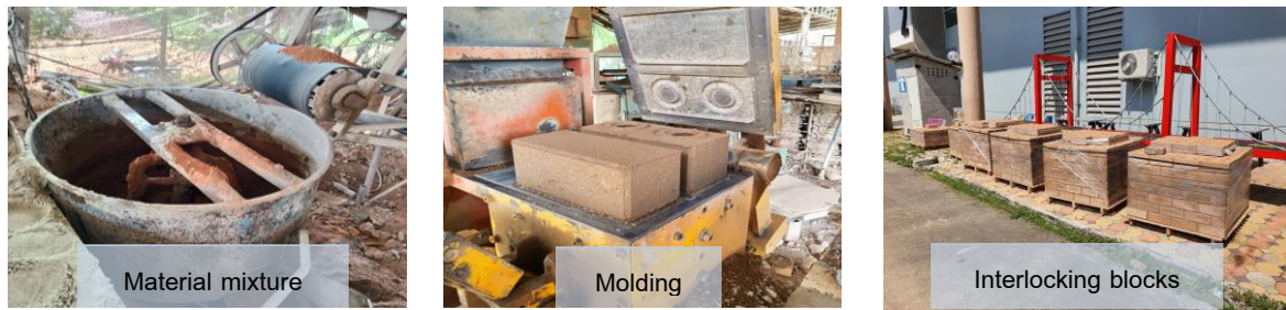
Figure 2 The molding of interlocking blocks with rubberwood ash mixture.
