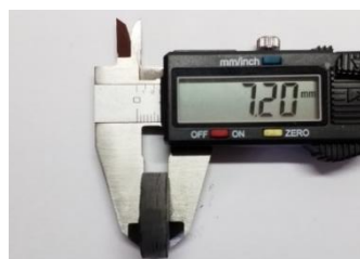
Figure 4 Appearance and dimensions of a sintered membrane
