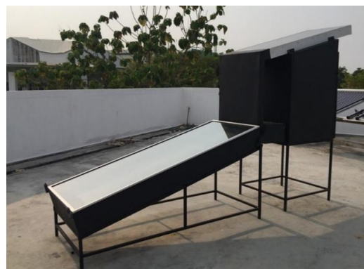
Figure 2 Photograph of the PVT-porous dryer.
