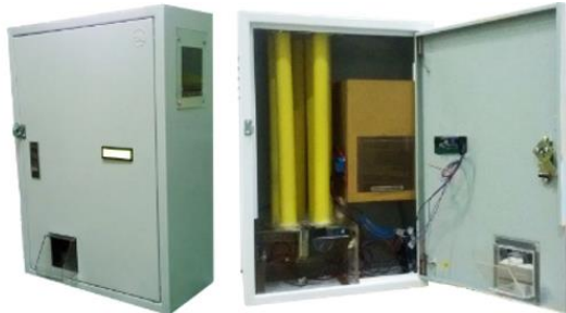
Figure 5 The proposed ten-baht coin swap machine
