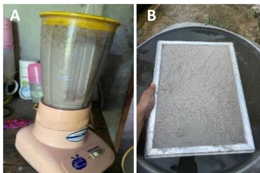
Figure 1 (A) Mixing of sugarcane paper pulp; (B) Sugarcane paper forming
