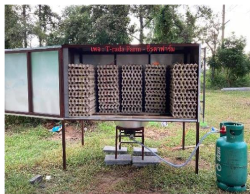
Figure 3 Disinfection of egg trays by steaming [9]
