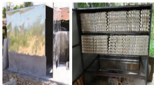
Figure 2 Disinfection of egg trays with hot air [8]
