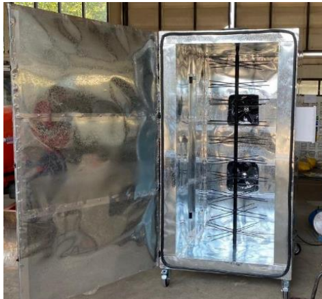
Figure 4 UV/hot air disinfection chamber for bacterial disinfection of egg trays
