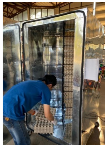
Figure 7 Loading egg trays in the UV/hot air disinfection chamber
