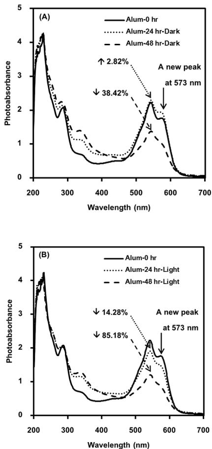
**Figure 4** Photo-absorbance of the chelated SE incubated under dark conditions (A) and light conditions (B)
