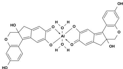
**Figure 2** Structure of  $Al(brazilein)_2$  complex from brazilein and aluminum (III) ion complexation [18]
