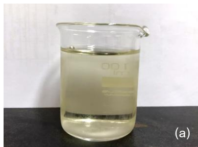
Figure 1. Materials (a) 10% W/V Polyaluminium chloride (PACI) (b) Water treatment sludge
