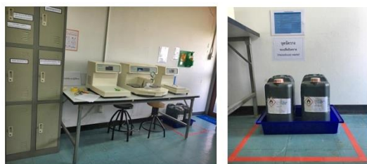
Figure 8. The appropriate waste container specifically for flammable chemical and stored away from heat, fire sources and flame (after the implementation)
