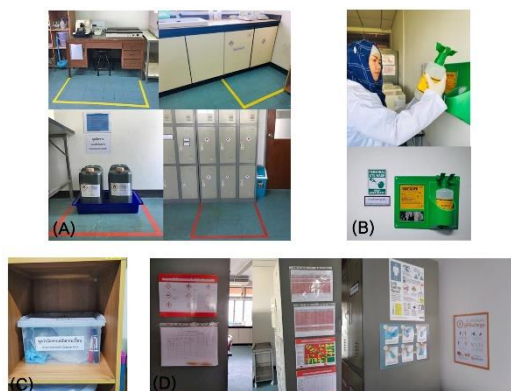
Figure 14. (A) Identification of working area: yellow tape for high risk area and red tape for extreme risk area, (B) Eye wash equipment and inspection, (C) The provision and putting up sign of location of chemical spill cleanup kits and (D) Putting up of several signs (after the implementation)
