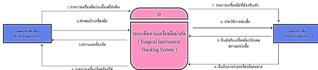
Figure 1. Context Diagram illustrating the operational scope of the Surgical Instrument Tracking System
