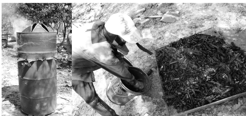
Figure 3 Burning wood chips from teak, mango and jackfruit in a 200 litter-barrel kiln (left) and bio-char products (right)
