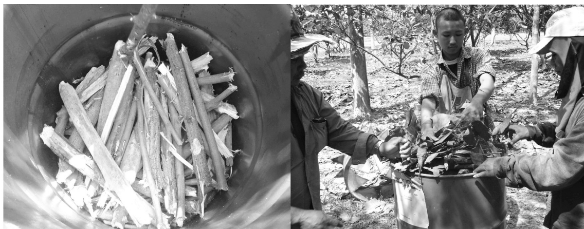
Figure 2 Wood chips from teak, mango and jackfruit were contained into 200 litter-barrel kiln (left) before leaves and small wood chips had been topped for fire easily (right)
