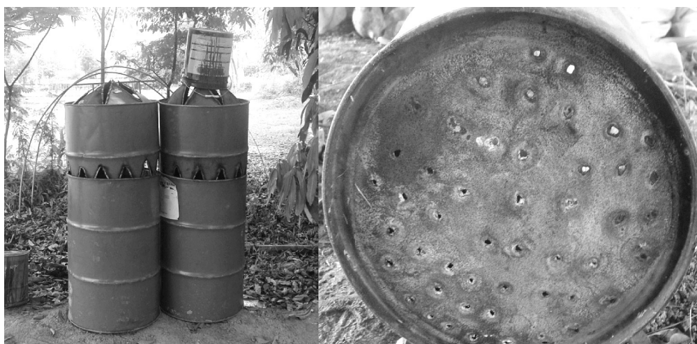
Figure 1 200 liter barrel were adapted to bio-char kiln
