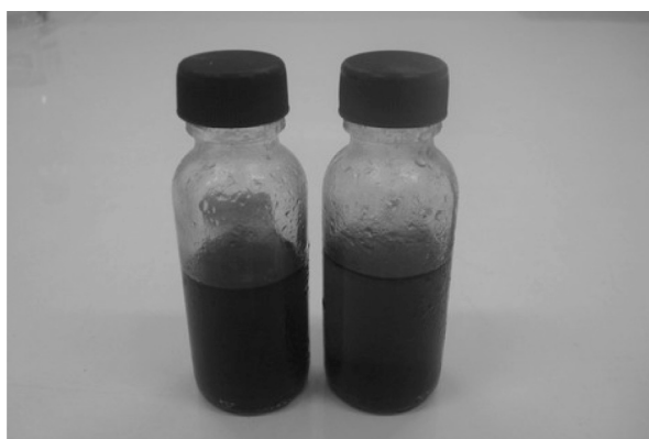
Figure 4 Bio-oil from Dry-ice/Acetone condenser
