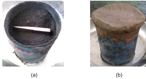
Figure 4 (a) A part of the big knife embedded in a carburizing box (b) The lid of the carburizing box was sealed using clay
