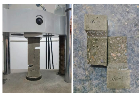
(a) GV Sample failure
