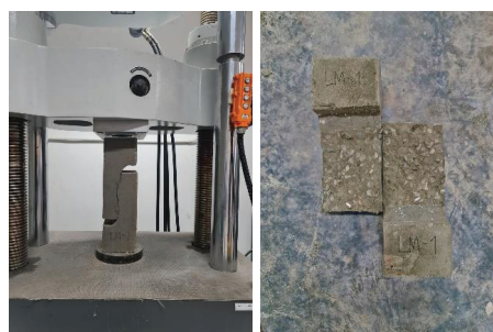
(b) LM Sample failure
