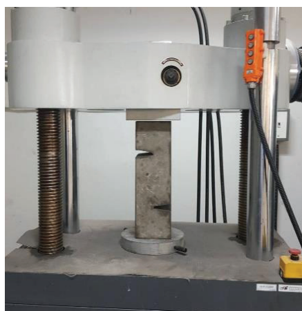
(b) Direct shear test on UTM
