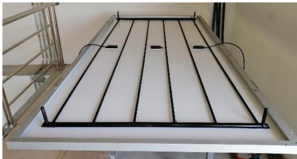
Figure 4 Heat sink under solar cell (Design)
