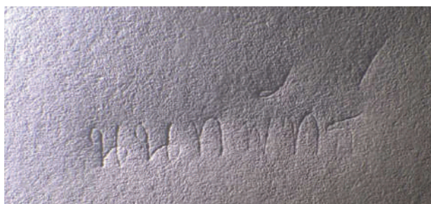
Figure 3 Image of the 1st paper backing using oblique light shining to the left, height 10 mm.
