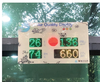
Figure 2 The air pollution sensor (AEROBOX) for measuring PM2.5
