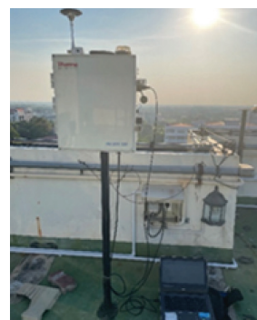
Figure 5 The Area Dust Monitor (ADR1500) for measuring PM2.5
