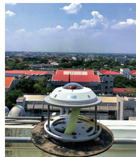
Figure 4 The sky camera for measuring cloud cover
