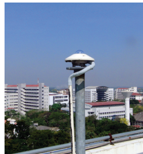
Figure 3 The pyranometer for measuring solar irradiance
