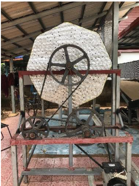
Figure 2 Reduce motor speed with pulley sets.
