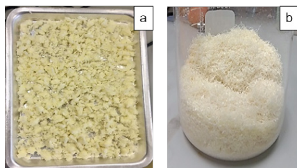
Figure 3 Characteristics of extracted cellulose (a) cellulose before drying and (b) cellulose after drying and milling.
