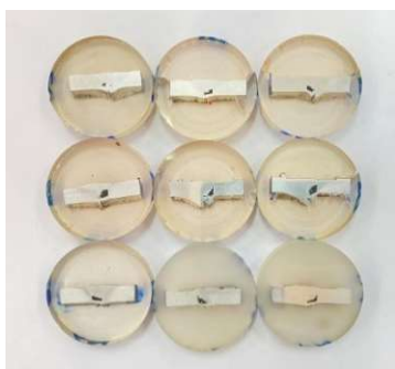
Figure 8 Cross section specimen ready for inspection
