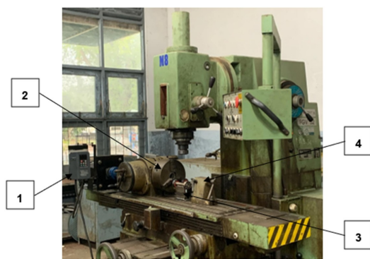
Figure 2 Friction stir welding machine for aluminum pipe work
