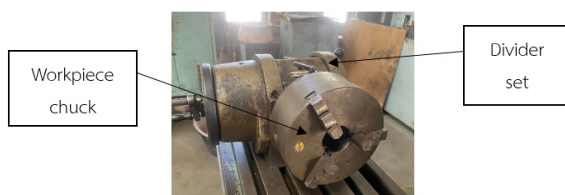
Figure 11 Equipment for holding pipe workpieces
