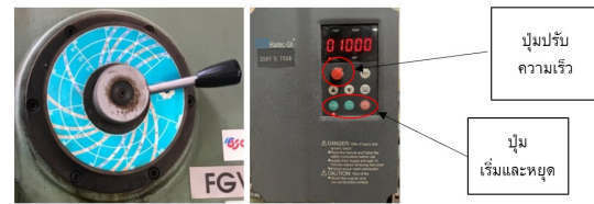
Figure 4 Adjusting welding rotation speed and welding travel speed
