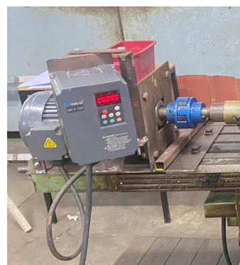
Figure 10 Layout of the welding speed control unit of the equipment
