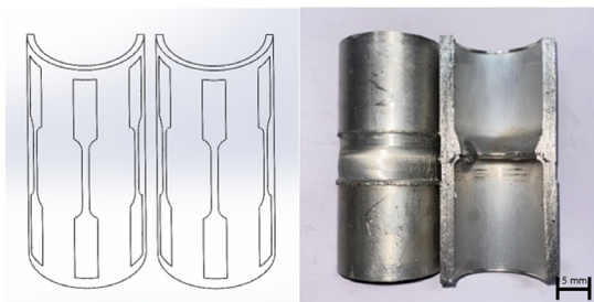
Figure 6 Layout and cutting of the workpiece
