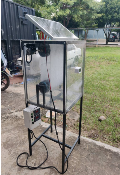
Figure 1 Solar-powered air purifier.
