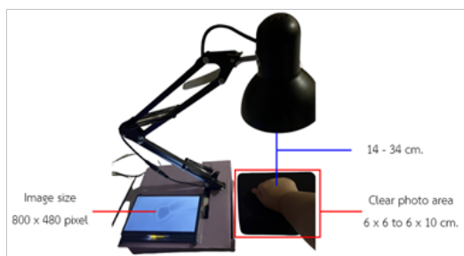
Figure 5 Diagram illustrating the operational principle of the device
