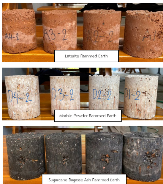
Figure 9 Erosion resistance test for specimens from local materials
