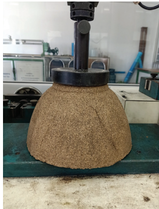
Figure 3 Plant pot mod from the cassava rhizome and bagasse by hydraulic machine
