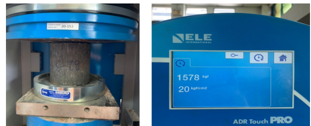
Figure 3 Compressive strength test
