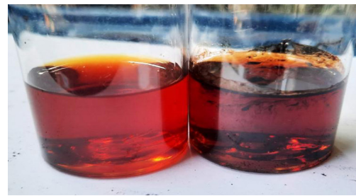
Figure 6 Wood vinegar obtained from traditional kiln (left) and 200-liter low-emission kiln (right)
