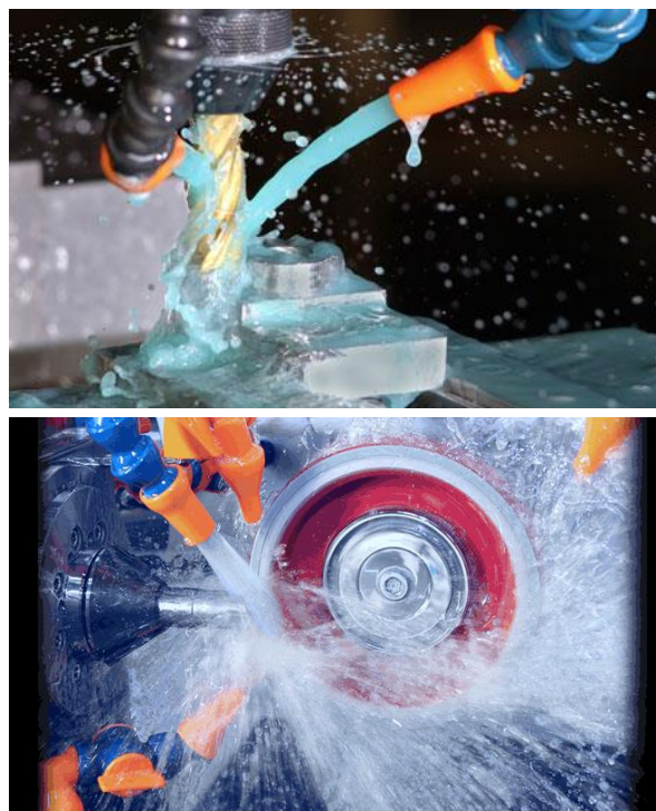
Fig. 1 a). Metalworking fluids employed in drilling process, b). in grinding process
