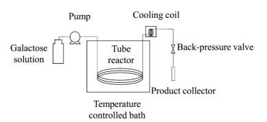
Figure 4 Schematic diagram of flow-type subcritical fluid treatment instrument for tagatose production.
