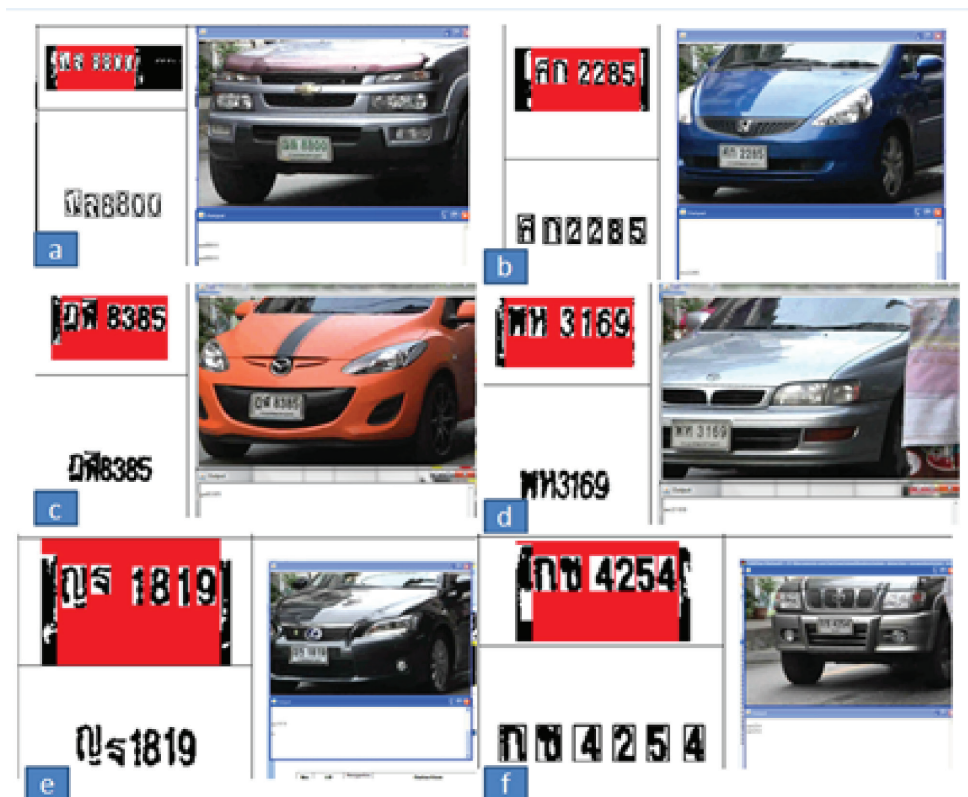
Figure 8 The TLPRS some successful license plate localization, segmentation and character recognition images
