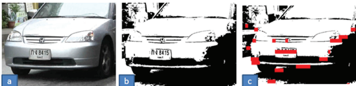
Figure 3 The TLPRS sample images (a) RGB video image, (b) B&W image, (c) all possible license plate rectangles.
