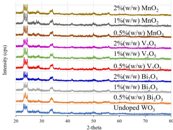
**Figure 2.** XRD patterns of Bi/V/Mn oxide doped WO<sub>3</sub>
