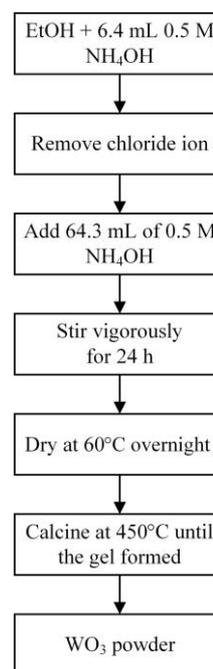
**Figure 1.** Photocatalyst preparation using sol-gel method
