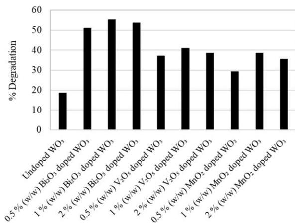
**Figure 4.** Degradation of S-metolachlor using Bi/V/Mn oxide doped WO<sub>3</sub> after 4 h under visible light
