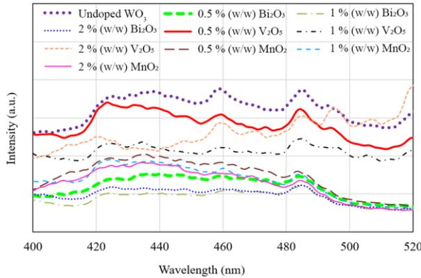
**Figure 3.** Photoluminescence spectrum of Bi/V/Mn oxide doped WO<sub>3</sub>
