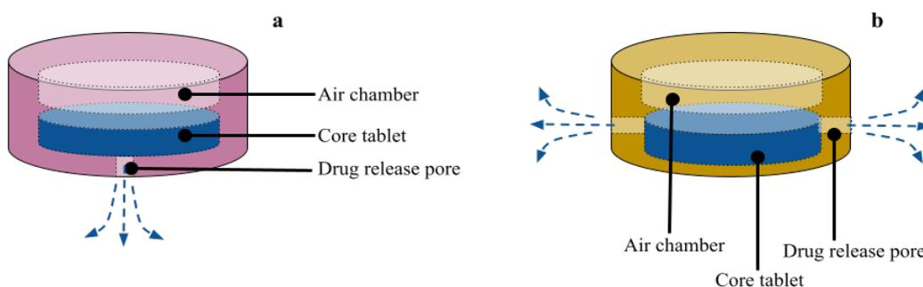
**Figure 6.** Schematic of 3D-printed floating drug delivery system with (a) zero-order kinetic drug release and (b) antiflip-up mechanism
