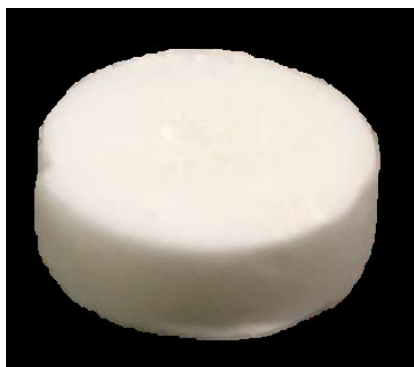
Figure 6. Image of piroxicam/HP \beta CD lyophilisates consisting of 0.8% w/w gelatin, 1.2% w/w HPMC, 1% w/w piroxicam, 2.5% w/w HP \beta CD, 0.2% w/w PEG400, 1% w/w erythritol, and 0.75% citric acid
