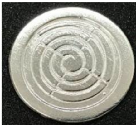
Figure 2. The silver disc test plate with a deeply embossed surface
