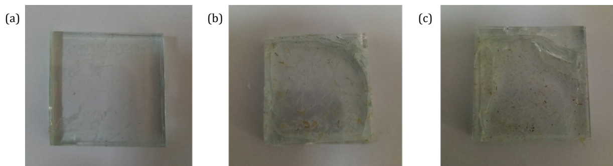
Figure 6. The physical appearance of a sandwich-structured glass after being subjected to stress. The interlayer part contained (a) epoxy, (b) epoxy and spikelet fiber with a size of 250 \mu\text{m} , and (c) epoxy and stalk fiber with a size of 250 \mu\text{m}
