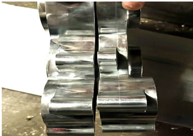
Figure 6. The machined & polished gearbox casing
