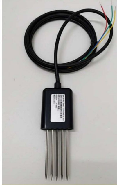
Figure 3. Atech sensor (NPK, pH, moisture, temperature, EC, RS485)
