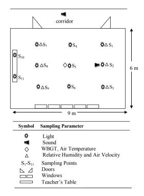
**Figure 2** Sampling points  $(S_1 - S_{11})$  within classrooms in this study. Due to time limitation and restriction of the number of instrument, sound level was measured only at the sampling point  $S_2$  in the middle of the last row at the back, which was assumed to be the least sound level compared with other rows in classrooms.
