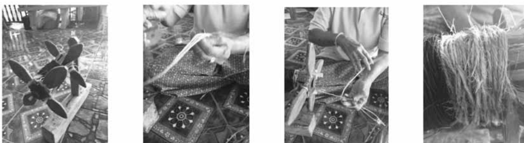
Figure 3 The process of spinning the stem into bundle fibers by hand
