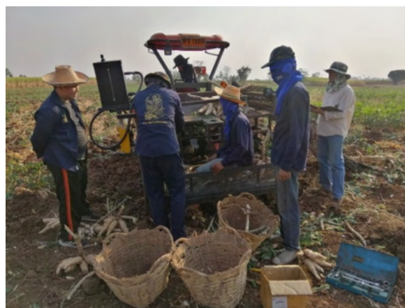
Figure 5 Testing conveyor and cutting machine attached to a tractor for harvesting cassava in the field
