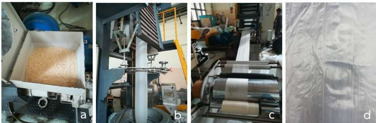
Figure 2 PBAT pellets for biodegradable plastic (a), blown film production form PBAT (b-c) and PBAT film (d) with its low melt flow rate, it is ideal for producing plastic with uniformity throughout the forming process
