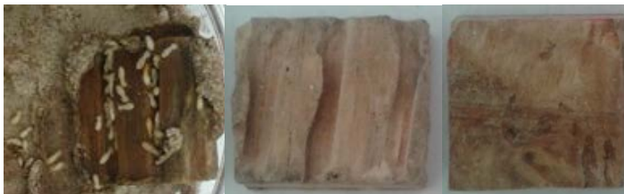
Figure 5 Subterranean termite infestation on rubberwood plywood produced with urea-formaldehyde adhesive (left), a destroyed rubberwood plywood produced with urea-formaldehyde adhesive after exposure to subterranean termite (center), and a destroyed rubberwood plywood produced with urea-formaldehyde adhesive with 10% borax loading content added after exposure to subterranean termite (right).
