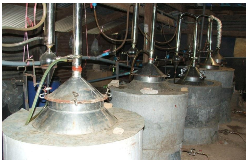
Figure 3 Distillation apparatus for agarwood oil extractives of farmers' Aquilaria plantation in Trat province.
