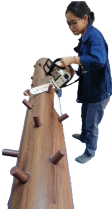
Figure 4 Depiction of a chainsaw delimbing time study.
