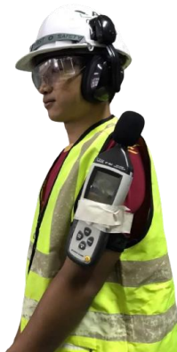
Figure 3 Installed sound measuring device on the operator.
