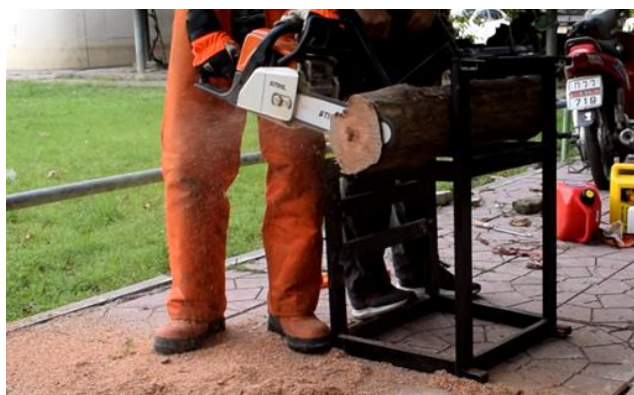
Figure 5 Setup to study the cutting speed.
