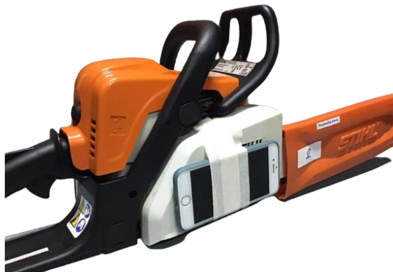
Figure 4 Installed device on the chainsaw for measuring vibration levels.
