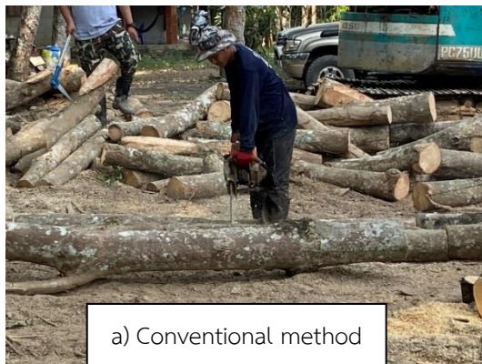
Figure 1 Bucking methods analyzed in the study a) conventional method and b) log supported method.
