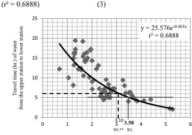
**Figure 8** Relationship between water level (WL) at the upper station (P82) and travel time (hr) of water from STA03 to STA04 that resulted in the maximum water level at STA04 (risk area).
