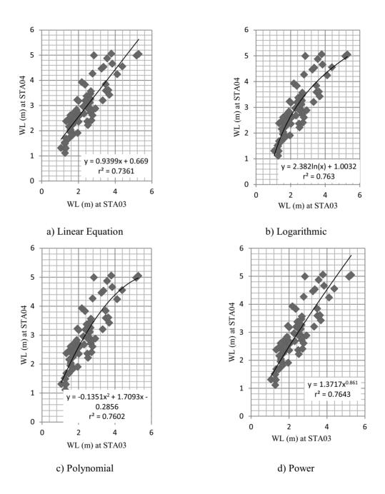
**Figure 6** Relationship of water level (WL) between two stations (STA03 and STA04) based on four equations.
