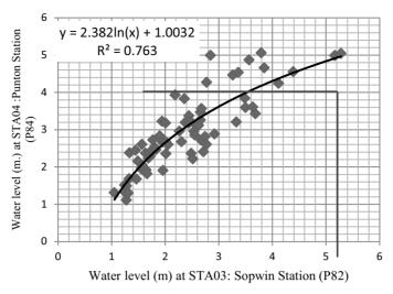
**Figure 7** Relationship between the water level at the upper station (STA03) and the lower station (STA04). The red line shows the level at STA04 (3.5 m) when the level at STA03 is 4 m.
