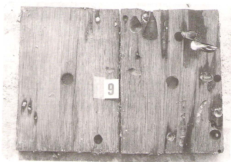
Figure 5. Shorea obtusa (No. 3) attacked by L. pedicellatus and Xylia kerrii (No. 9) by M. striata . Treated blocks (left), untreated (right) after nine month exposure.
