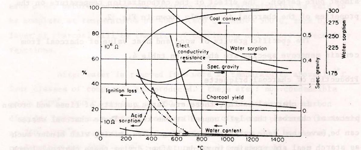
Figure 2. Effect of temperature on charcoal properties.
