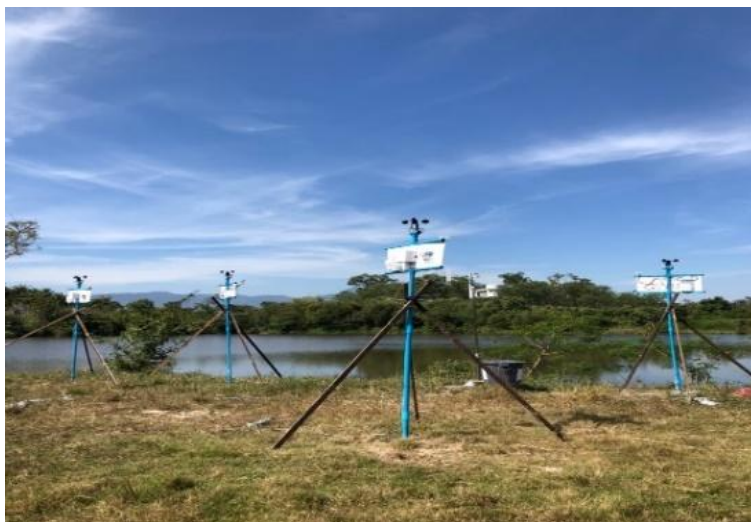
Figure 5 Testing the IoT weather Monitoring devices at the Had Wanakorn Forestry Research and Student Training Station
