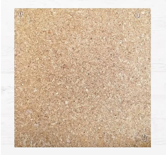
Figure 1 Particleboard made from teak sawdust
