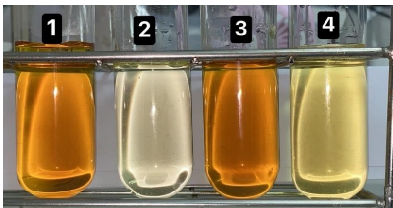
Figure 9 Appearance of iodine solution centrifuged for 3 minutes with 2 g of granular biochar (1), 700 °C-treated biochar with steam (2), treated biochar with plasma (3) and 700 °C treated biochar with steam + treated biochar with plasma, with 25 mL of test iodine solution
