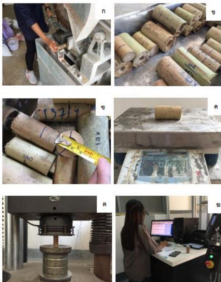
Figure 5 Mechanical properties (compression test of wood parallel to grain) a: cut samples b: samples that was cut c: volume measurement d: weight e: compression measurement f: record the highest compression.
