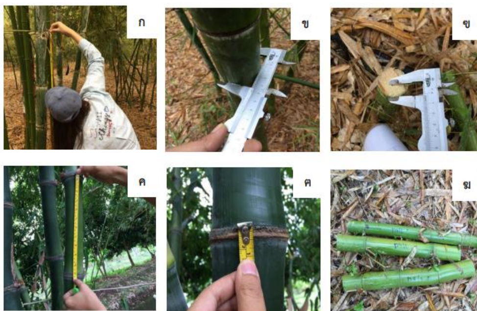
Figure 2 Determined bamboo sang mon clones that had good qualities to select good physical qualities clone. a: measured trunk length b: measured diameter c: measured wood thickness d: measured internode length e: measured joint length f: collected sample.
